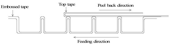
4.2 Embossed tape should not adhere to top tape when top tape is peeled back, and peel back direction is as follows.
